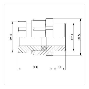
AF / OD [mm]: 22 Color: Gray Material: PA 6.0 Material Group: Plastic Mounting Hole [mm]: 19 Panel Thickness Range [mm]: 6.0-9.0 Protection Code: IP54 Thread Size: PG11 Weight: 8.98g Conformities:
