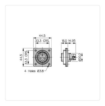
Amperage [A]: Color: Black Protection Code: IP68 Weight: 32g Conformities:
