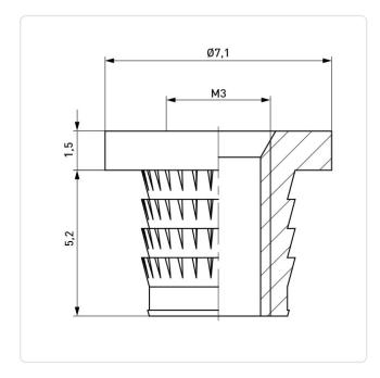
Finish: Plain Head Diameter [mm]: 7.1 Length [mm]: 5.2 Material: Brass Material Group: Brass Minimum Edge Distance [mm]: 1.7 Panel Hole Ø [mm]: 4 Thread Size: М3 Weight: 0.66g Conformities:
