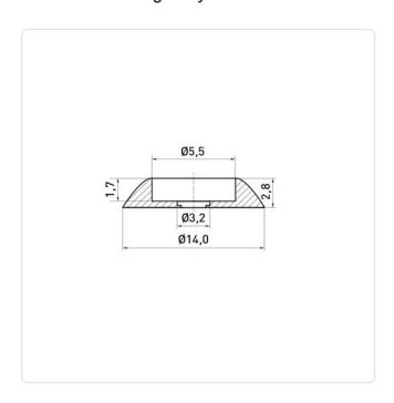
Color: Black For Thread Size: МЗ Height [mm]: 2.8 Inner Diameter [mm]: 3.2 Material: PA 6.0 Material Group: Plastic Outer Diameter [mm]: 14 Weight: 0.32g
