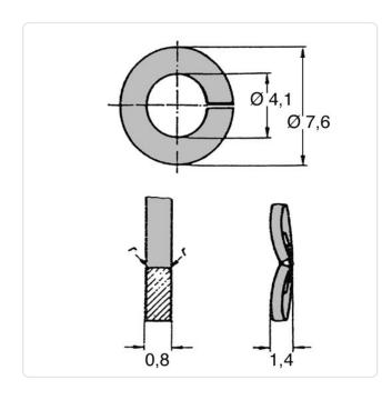
DIN/ISO: DIN128A Finish: Plain For Thread Size: M4 8.0 Height [mm]: Inner Diameter [mm]: 4.1
