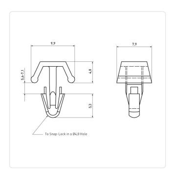
Color: Natural Flammability Class: UL94-V2 Head Diameter [mm]: 9.9 PA 6.6 Material: Material Group: Plastic
