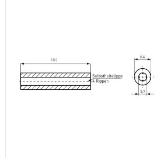
Color: Gray Flammability Class: UL94-V0 For Thread Size: M3 Inner Diameter [mm]: 3.7 Length [mm]: 10 Material: PVC - Polyvinyl Chloride Material Group: Kunststoff Outer Diameter [mm]: 6.4 Weight: 0.32g Conformities: Reach RoHS SVHC
