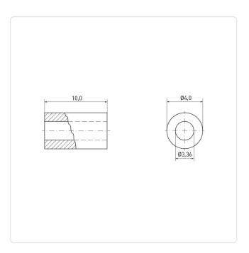
Finish: Plain Inner Diameter [mm]: 3.36 Length [mm]: 10 Material: Copper Material Group: Copper Outer Diameter [mm]: 4.04
