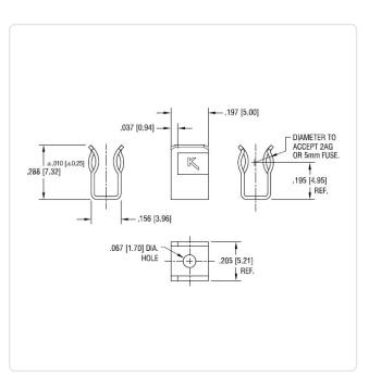
Amperage [A]: 15 Fuse Size [mm]: 5.0x20.0 Material: **Brass** Material Group: **Brass**
