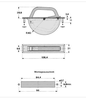
Black Color: Dist. Mounting Holes [mm]: 96 Height [mm]: 21 Material: PA 6.0 25% GF Material Group: Plastic Model: **Carrying Handle** Width [mm]: 106.4 33g Weight: Conformities: Reach RoHS SVHC
