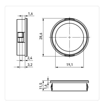
Color: Black Inner Diameter [mm]: 19 Material: PA 6.6 Material Group: Plastic Max. Panel Thickness [mm]: 3.2 Mounting Hole [mm]: 25.5 Weight: 2.13g Conformities:
