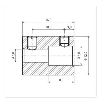
Height [mm]: 16 Inner Diameter [mm]: 6 Material: **Brass** Material Group: Brass
