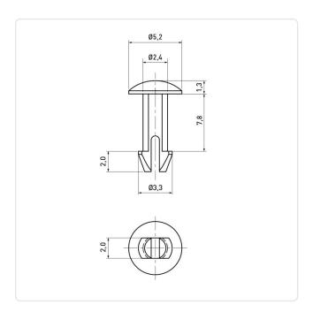
Color: Natural Flammability Class: UL94-V2 Head Diameter [mm]: 5.2 Material: PA 6.6 Material Group: **Plastic** Mounting Hole [mm]: 2.4 Weight: 0.08g
