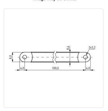
Insulation: Polyolefin 108 Length [mm]: Material: Copper Material Group: Copper Mounting Hole [mm]: 3.2
