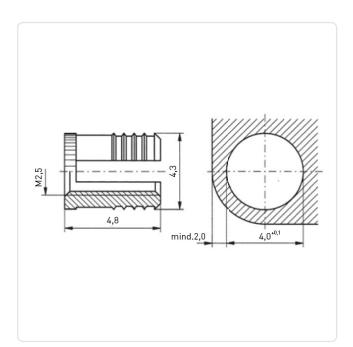
Finish: Plain 4.8 Length [mm]: Material: Brass Material Group: Brass Minimum Edge Distance [mm]: 2.0 Panel Hole Ø [mm]: Thread Size: M2.5 Weight: 0.28g
