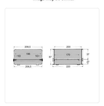
Color: Blue Height [mm]: 67 Length [mm]: 220 Material: Steel Material Group: Steel Width [mm]: 208.5 Weight: 1049g Conformities:
