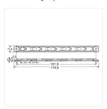
Color: Black Dist. Mounting Holes [mm]: 161.9 Flammability Class: UL94-V2
