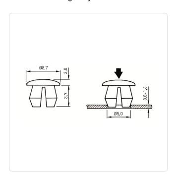
Color: Natural Inner Diameter [mm]: 4.8 Material: PA 6.6 Model: Hole Plug Outer Diameter [mm]: 8.7
