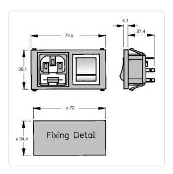
Amperage [A]: 10 Color: Black Connections: 6.3x0.8 Fuse Size [mm]: 5.0x20.0
