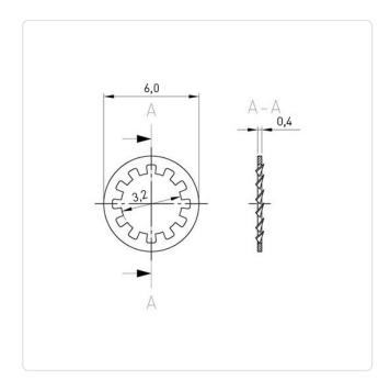
DIN/ISO: **DIN6797I** Finish: Plain For Thread Size: M3 0.4 Height [mm]: Inner Diameter [mm]: 3.2
