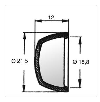
Color: Black Head Height [mm]: 12 Inner Diameter [mm]: 18.8 PA 6.0 Material: Material Group: **Plastic**
