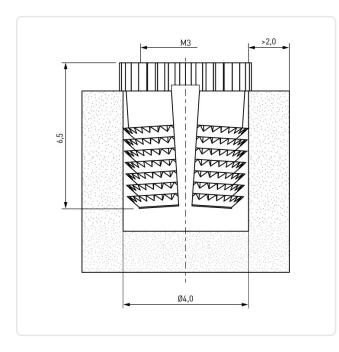
Finish: Plain Length [mm]: 6.5 Material: **Brass** Material Group: Brass Minimum Edge Distance [mm]: 2.0 Panel Hole Ø [mm]: 4 Thread Size: М3 Weight: 0.29g
