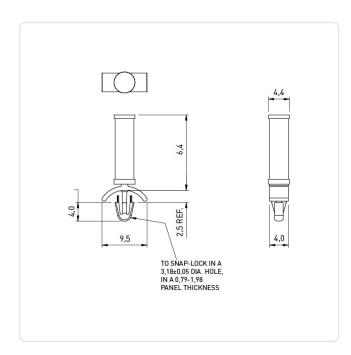
Color: Natural Flammability Class: UL94-V2 Length [mm]: Material: PA 6.6 Material Group: **Plastic** Panel Hole Ø [mm]: 3.2 Panel Thickness [mm]: 0,8-2,0
