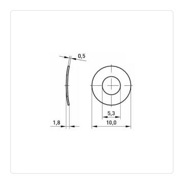
DIN/ISO: DIN137A Finish: Plain For Thread Size: M5 0.5 Height [mm]: Inner Diameter [mm]: 5.3
