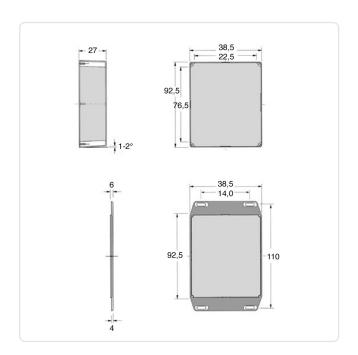
Height [mm]: 27 92.5 Length [mm]: Material: Aluminum Material Group: Aluminum Protection Code: IP54 Width [mm]: 38.5
