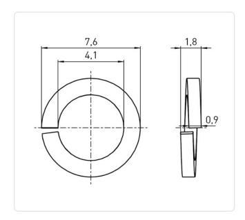
DIN/ISO: DIN127B Finish: Plain For Thread Size: M4 0.9 Height [mm]: Inner Diameter [mm]: 4.1
