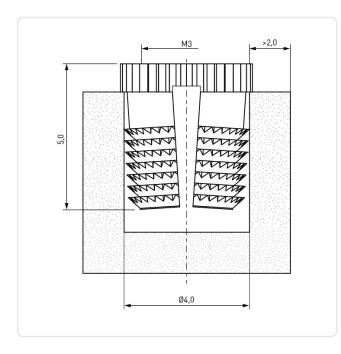
Finish: Plain Length [mm]: 5 Material: **Brass** Material Group: Brass Minimum Edge Distance [mm]: 2.0 Panel Hole Ø [mm]: 4 Thread Size: М3 Weight: 0.24g
