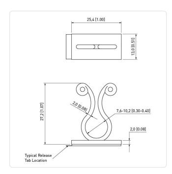
Bundle Diameter [mm]: 3,0-10,0 Color: Natural Flammability Class: UL94-V2 PA 6.0 Material: Material Group: **Plastic**
