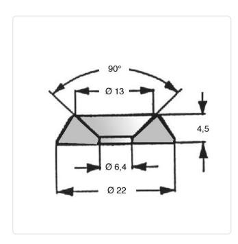
Color: Black For Thread Size: M6 Height [mm]: 4.5 Inner Diameter [mm]: 6.4 Material: PA 6.0 Material Group: Plastic Outer Diameter [mm]: 22 Weight: 1.17g
