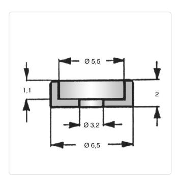
Color: Black For Thread Size: МЗ Height [mm]: Inner Diameter [mm]: 3.2 Material: PA 6.0 Material Group: Plastic Outer Diameter [mm]: 6.5 Weight: 0.05g
