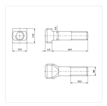
DIN/ISO: **DIN787** Plain Finish: Head Height [mm]:
