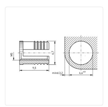
Finish: Plain Length [mm]: 9.5 Material: Brass Material Group: Brass Minimum Edge Distance [mm]: 3,2 Panel Hole Ø [mm]: 6.5 Thread Size: M5 Weight: 0.95g
