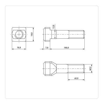
DIN/ISO: **DIN787** Finish: Plain Head Height [mm]:
