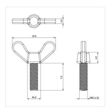
Color: Natural Flammability Class: UL94-V2 Head Diameter [mm]: 20 Length [mm]: 9.5 Material: PA 6.6
