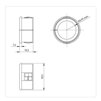
Color: Black Inner Diameter [mm]: 14 Material: PA 6.6 Material Group: Plastic Max. Panel Thickness [mm]: 3.2 Mounting Hole [mm]: 19.1 Outer Diameter [mm]: 19.8 Weight: 0.85g
