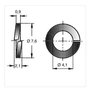
DIN/ISO: DIN127B Finish: Plain For Thread Size: M4 0.9 Height [mm]: Inner Diameter [mm]: 4.1
