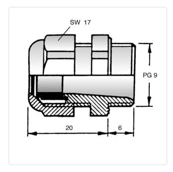
AF / OD [mm]: 17 Material: **Brass** Material Group: **Brass** Mounting Hole [mm]: 15.7 Panel Thickness Range [mm]: 4.0-8.0 Protection Code: IP68 Thread Size: PG9 Weight: 17.41g
