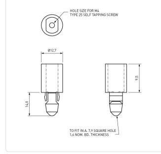
Color: Natural Flammability Class: UL94-V2 Length [mm]: 9.5 PC - Polycarbonate Material: Material Group: Plastic Panel Hole Ø [mm]: 7.9 Panel Thickness [mm]: 1,6 Weight: 1.4g Conformities: Reach RoHS SVHC
