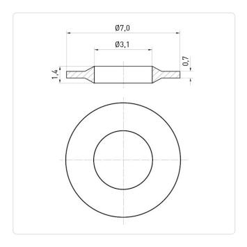
For Thread Size: М3 1.4 Height [mm]: Inner Diameter [mm]: 3.1 Material: PA 6.0 Material Group: **Plastic** Outer Diameter [mm]: 7
