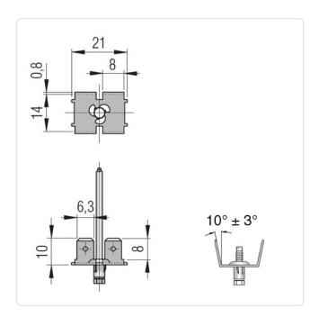
Bending Angle [°]: 10 Finish: Plain Material: **Brass** Material Group: **Brass** Mounting Hole [mm]: 5.2 Panel Thickness [mm]: 0,6-2,0 Plug-In Length [mm]: 7.8 Size [mm]: 6.3x0.8 Tabs: 4 Weight: 5.64g Conformities:
