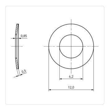
DIN/ISO: **DIN2093** Finish: Plain For Thread Size: M6 0.5 Height [mm]: Inner Diameter [mm]: 6.2
