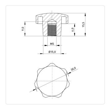
Color: Black Diameter [mm]: 30 Height [mm]: Material: PA 6.0 Material Group: Plastic Thread Size: M5 Weight: 9.4g
