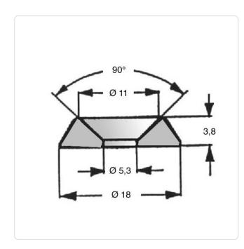
Color: White For Thread Size: M5 Height [mm]: 3.8 Inner Diameter [mm]: 5.3 Material: PA 6.0 Material Group: Plastic Outer Diameter [mm]: 18 Weight: 0.7g
