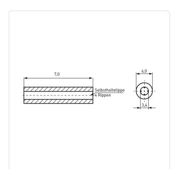
Color: Black Flammability Class: UL94-V2 For Thread Size: М3 Inner Diameter [mm]: 3.4 Length [mm]: 7
