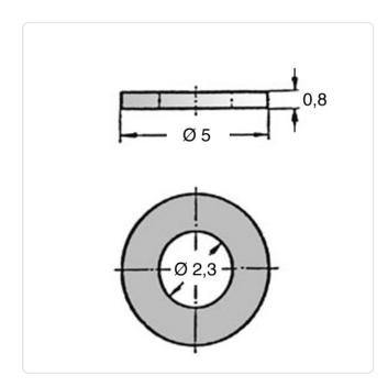
Color: Russet For Thread Size: M2 Height [mm]: 8.0 Inner Diameter [mm]: 2.3
