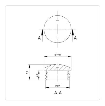
Color: Black Height [mm]: 9 Material: PA 6.0 Material Group: Plastic Model: Plug Screw
