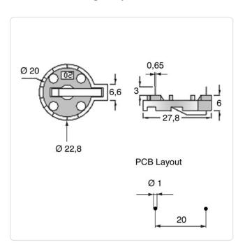
Battery Type: Cell Dia. 20mm
