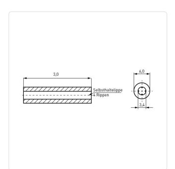
Color: Black Flammability Class: UL94-V2 For Thread Size: М3 Inner Diameter [mm]: 3.4 Length [mm]:
