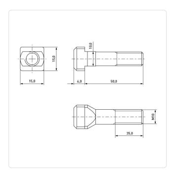
DIN/ISO: **DIN787** Finish: Plain Head Height [mm]:
