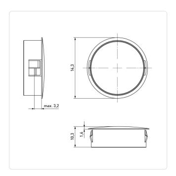
Color: White Flammability Class: UL94-V2 Head Diameter [mm]: 14.7 Head Height [mm]: 1.6 PA 6.6 Material: Material Group: Plastic Snap-In Model: Mounting Hole [mm]: 12.7
